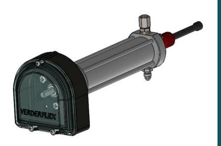
An electric dosing system using a peristaltic pump driven by a brushless dc motor/gearbox assembly specifically matched to the pump drive speed requirement. Motor speed/pumping rate controlled by serial command.
